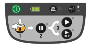
The **ON/OFF** ① button is in the top left of the Control Panel in the gray bar. Push and hold this button for one second to power up or power down the LUCAS device. When the device powers up, it automatically does a self-test of the functions and the protective system. When the self-test is complete, the green LED beside the **ADJUST** ③ key illuminates. This takes approximately three seconds.
