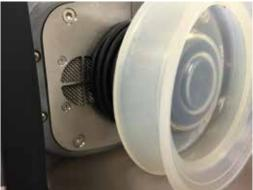
Underneath the Hood is the Piston, which contains the Pressure Pad and the Suction Cup.
